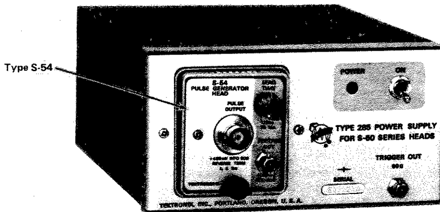
(C) Installed in Type 285 Power Supply Compartment
